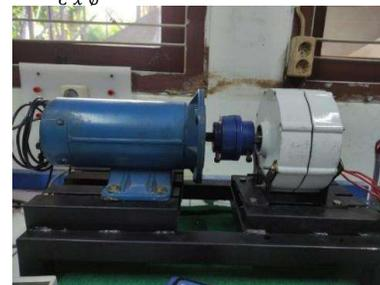
Gambar. 4 *DC Motor 180V DC Magnet Permanent*
